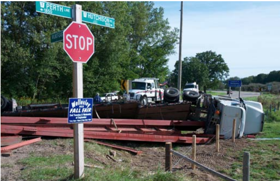
This roll over carried a potentially deadly load of steel girders, which were spewed across a 75-metre swath as it crossed the T-intersection. In this instance, if an other vehicle had come to a stop and then edged past this stop sign, it would have been in the path of the on-coming girders. Note the fence.
